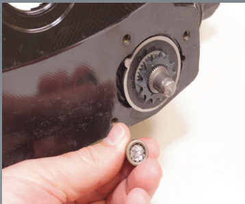
Failed adjuster / Requires caliper replacement
