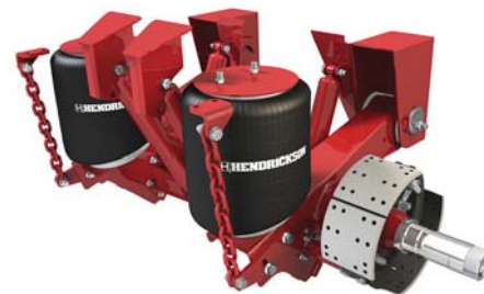
AAEDT 30K with optional chain down-stops and rear-mount shocks
