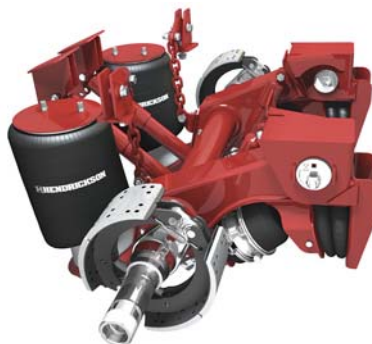
AAEDL 30K with optional chain down-stops, rear-mount shocks and UNDER BEAM LIFT™ (UBL™)
