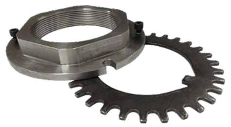
The SKF spindle nut locking system offers a new, robust and affordable lock nut system for tractors and trailers alike. Forged, precision machined and assembled with two high-strength lock bolts, the SKF spindle nut locking system yields one of the strongest systems available today. Coupled with the precision stamped lock washer, this system provides the user with end-play adjustability that exceeds the stringent demand of today's field environment and maintenance requirements.
